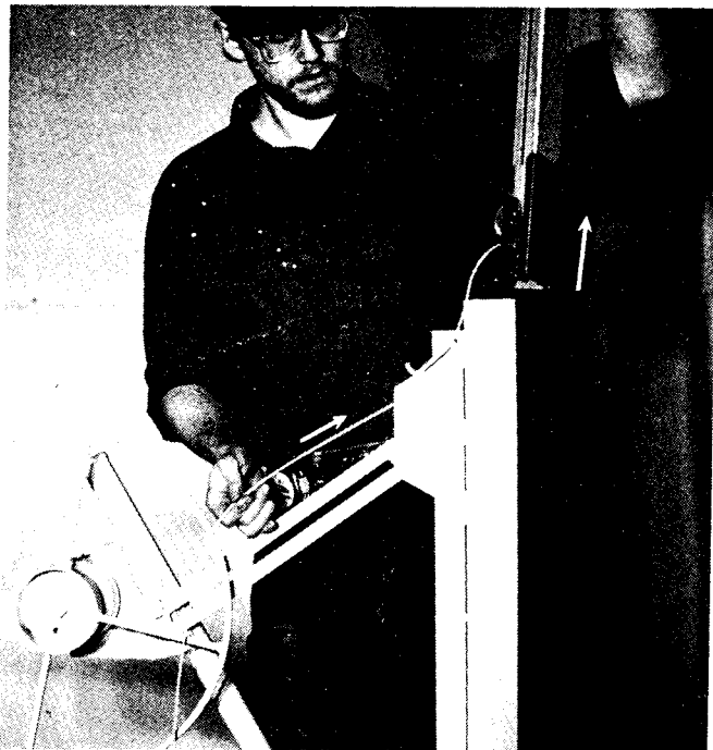
3. Remove the two telescoping sections completely from the frame housing. Pull the cable out with them.
