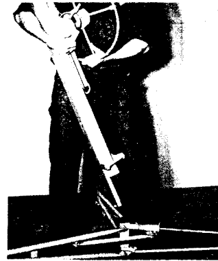
9. Lift the frame off of the tripod base.
