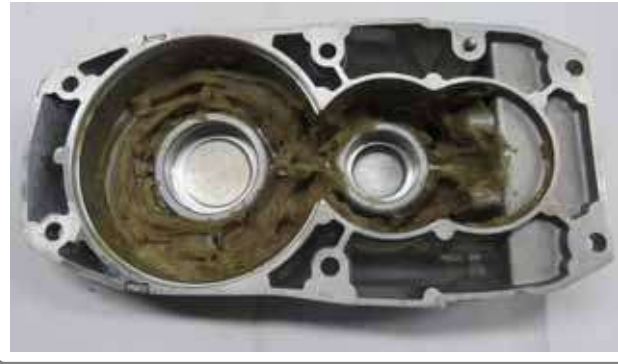
Fig. 12 • Gear cover filled with Nippeco SEP-3A grease
